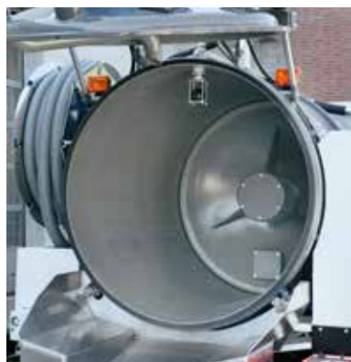
Movable partition for capacity increases, only for Flexcom 10 or 12 tonnes.
